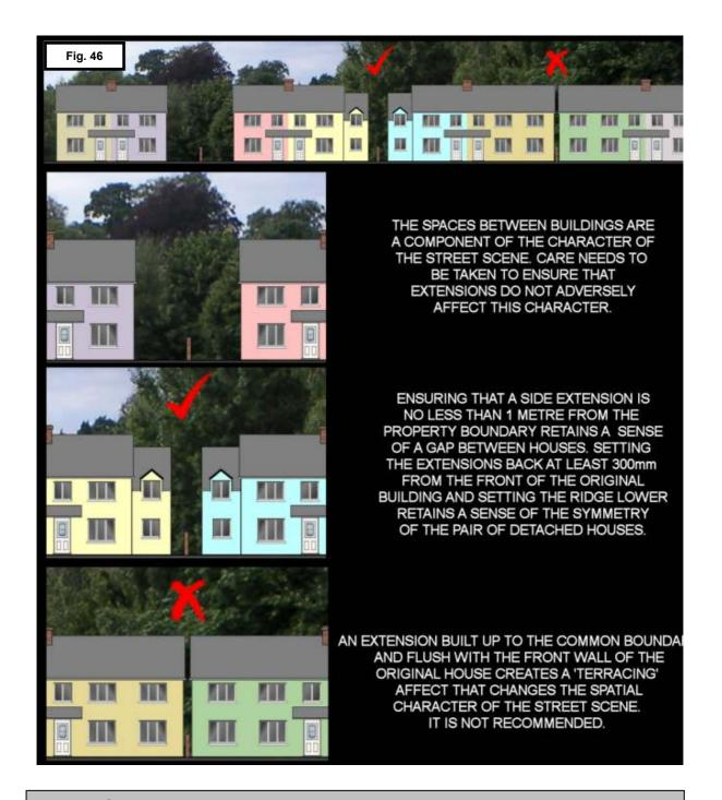
6.10 NOTE 17: A side extension to a semi-detached property should respect the original symmetry of the pair of buildings. (EV45)
