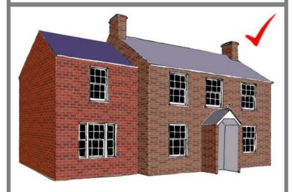
By setting the extension back from the face of the building the change of material is made less jarring and the symmetry of the original building is respected.
