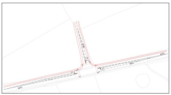
Figure 4.3 – Indicative Site Access Arrangement (3-arm junction)
