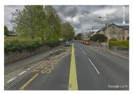
Image 12 – Pedestrian crossing with tactile paving, dropped kerbs, reduced crossing width and protective bollards. (© Google Streetview 05/18)
