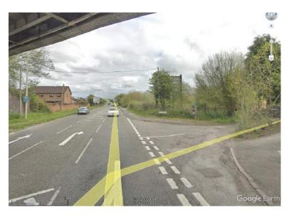
Image 24 - Missing dropped kerbs and tactile paving at Hernston Lane junction (© Google Streetview 05/18)
