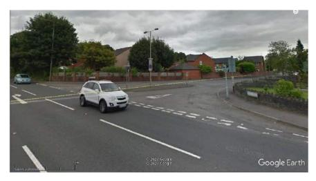
Image 5 – No dropped kerbs and tactile paving crossing. (© Google Streetview 08/16)
