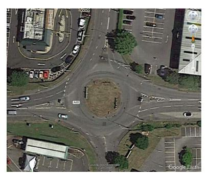
Image 26 – Pedestrian refuge islands with tactile paving and dropped kerbs on north, east and west arms of Picton Court Roundabout. Missing tactile paving on southern arm (© Google Satellite 6/25/2018)
