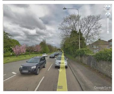
Image 22 – Street lighting present. Footway narrows on southern side of A48. There is potential scope for widening to create a shared pedestrian/cycle route (© Google Streetview 05/18)
