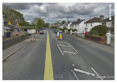
Image 10 – Pedestrian refuge island crossing with tactile paving and dropped kerbs. (© Google Streetview 05/18)
