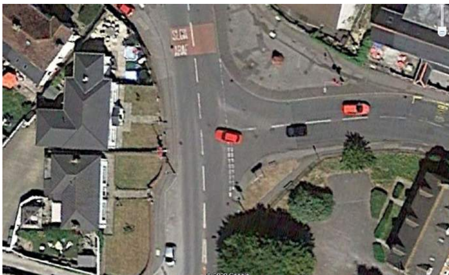
Image 6 – Missing dropped kerbs and tactile paving on School Terrace/Porthcawl Rd junction (© Google Satellite 6/27/2018)
