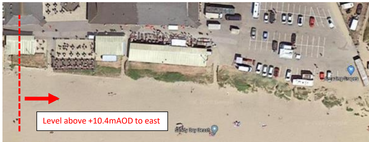
Figure 34: Aerial view of Sub-frontage 3 showing raised ground level (imagery ©2020 Google Maps)
