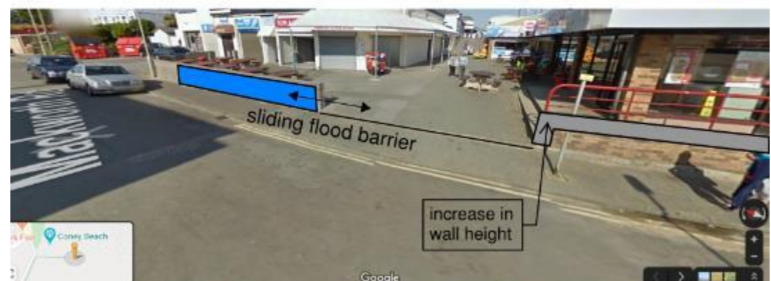
Figure 32: Concept of setback defence across opening on east of Mackworth Road (imagery ©2020 Google Maps)
