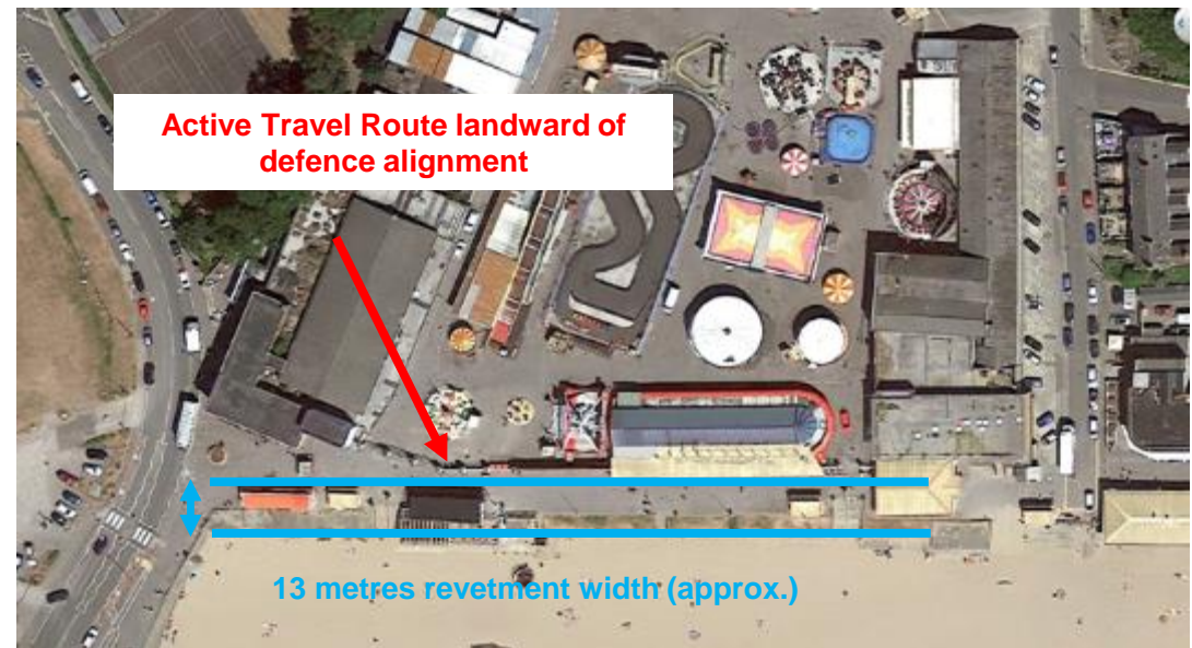
Figure 16: Width of revetment displayed on plan views (extract of LDP and aerial) (imagery ©2020 Google Maps)
