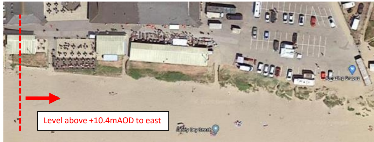
Figure 35: Aerial view of Sub-frontage 3 showing raised ground level (imagery ©2020 Google Maps)
