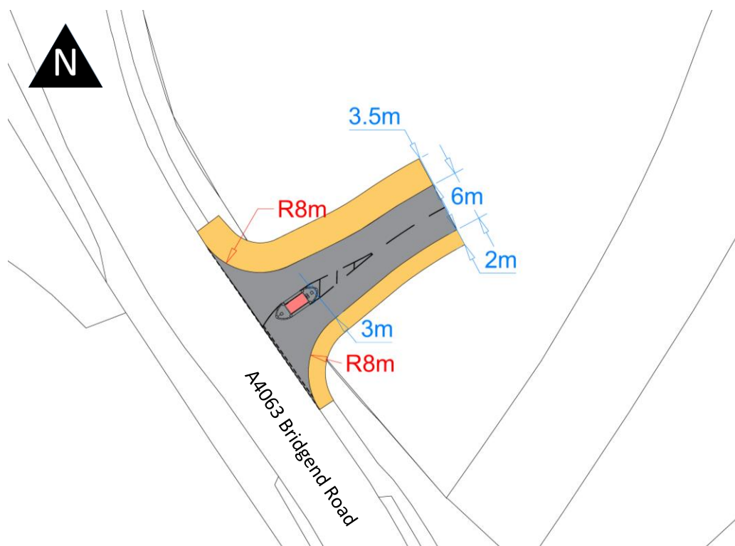
Figure 3.1 Site access on to the A4063 Bridgend Road
