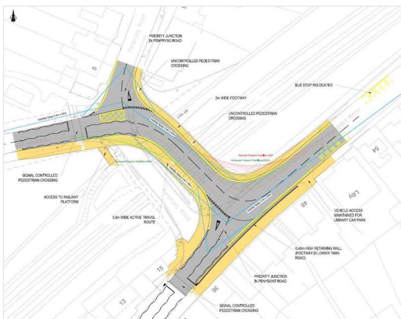
Figure 4: Option 6a (3-lane road bridge)
