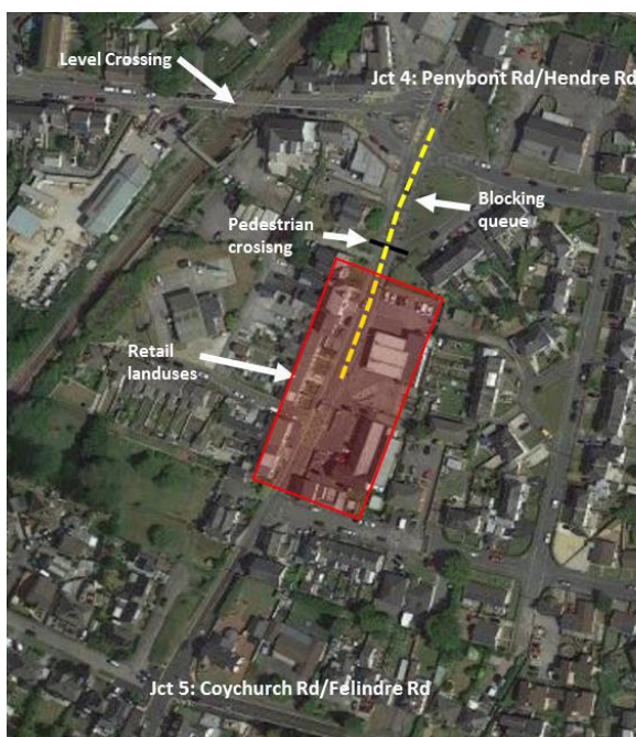
◀ Figure 2: Queueing on Coychurch Road Impeding Hendre Road Junction
